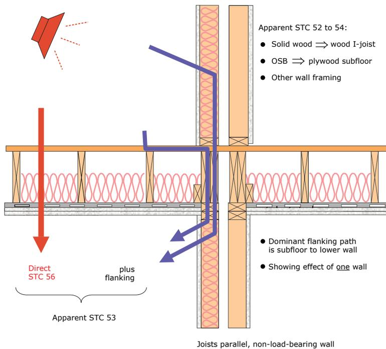
*Note: the red arrow indicates the direct path, and blue arrows indicate the flanking path*
