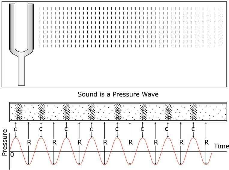
Note: In this figure, C signifies regions of compression and R signifies regions of rarefaction of the air molecules. Furthermore, the “0” pressure line in the graph represents the atmospheric pressure level.
